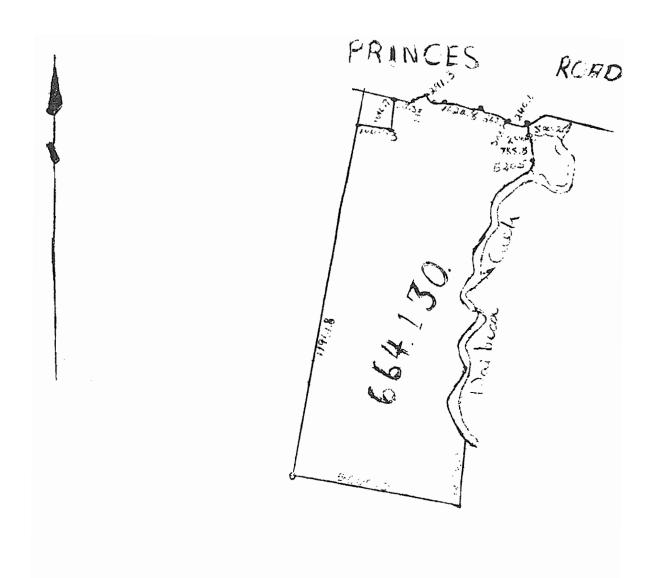
Scale 32 chains per inch. All measurements are in links.
