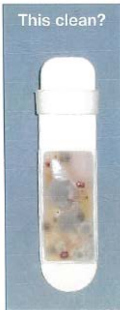
Swab No. 8 Cleaned Support chair Staphylococcus: Not present Streptococcus: Not present E. coli: 10 colonies Mould / Yeast: Heavy mould contamination Aspergillus, Penicillium and unknown mould
