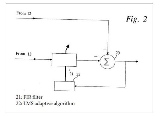
11 The Transversal filter shown in fig 2.1 of DAR11 is described in the associated text as an FIR transversal filter. The report says that the output of the FIR transversal filter is given by,
