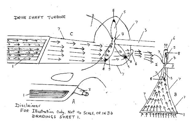
8 In the drawing, the turbine has a number of blades 5 with weighted tips 8 and is attached to the drive shaft 3 via the free-wheeling geared bearing 4. Air is introduced to the turbine through vents 1 via the air chamber 7. The pressure jet 6 is at the rear of the chamber.
