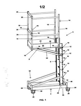
The apparatus is such that, in use, base 4 is positioned underneath platform 8
