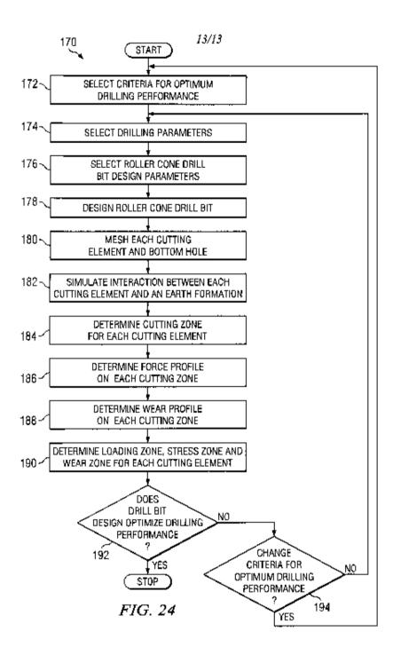
8 The first step is to select one or more drilling performance criteria that the designer is seeking to optimise. This might for example be the drilling life of the drill bit. Various drilling parameters are then selected (step 174). These may include for example diameter of the wellbore, speed of rotation of the drill bit, type of material being drilled. Various roller cone drill bit design
