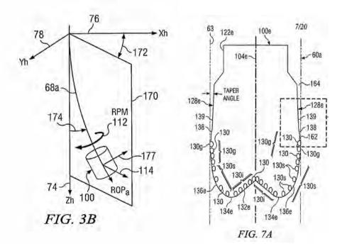
79 The design method subdivides the drill bit into inner and shoulder cutting zones (130i and 130s in figure 7A shown above) and also active and
