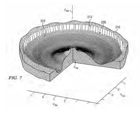
10 The mesh analysis enables the interactions of each cutting element with the downhole formation to be simulated (step 182). From this simulation it is possible to identify the mesh segments of the cutting element that will contact the formation during any discrete drilling period. This represents the cutting zone of the element (area indicated as 84 in figure 9). The core cutting zone is those segments of the mesh that contact the formation most of the time (shown as 84a).
