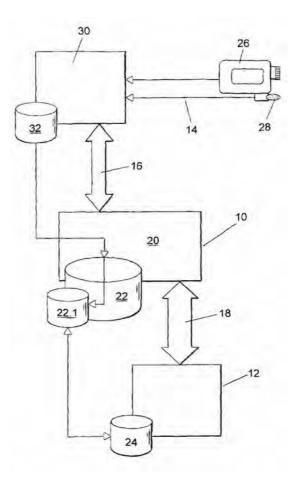
"The audio and/or visual recorder is constituted by a combination of a video camera 26, a microphone 28 and a laptop PC 30. The laptop PC 30 contains a data store 32. The recorder assembly 14 is adapted to convert the images and sounds recorded by means of the video camera 26 and the microphone 28 into digital data that is stored on the hard disk 32 of the PC 30.
