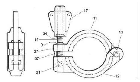
the bolt 15 can be swung between the prongs into the vertical position (as shown) and nut 17 tightened to hold the clamp shut.
