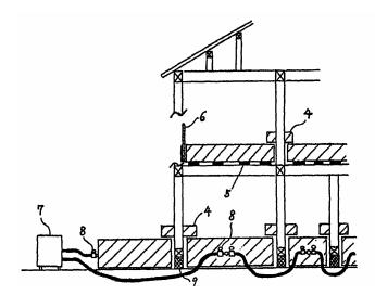
in which an accompanying list identifies the hatched sections as the airbag units, item 7 as an air compressor and items 8 as valves. Beyond a statement in section (3) of the description "Multiple numbers of units as described above combined together or used on their own along with an attached air compressor can be used as a system of preventing accidents involving people falling", there is no explanation of how the valves and the lines to them from the air compressor are arranged and operated.
