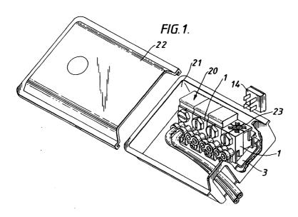
specification, shows a pole top distribution point incorporating the invention. It includes a number of connector units - four in this drawing - each connecting a pair of exchange wires with a pair of drop wires and all mounted on a common rail 3. There is a plug-in unit 14 on top of each connector unit. The whole assembly is enclosed in a weatherproof box 21.
