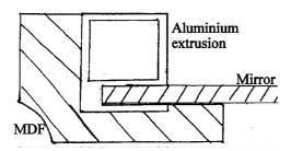
From the front of the wardrobe, the style appears to be made of medium density fibreboard (MDF). However this on its own would not be rigid enough, so it is stiffened by an aluminium extrusion having a box section portion with an L-shaped extension on the front side. The central panel - in this instance, a mirror - is held between the main box section and one arm of the extension.
