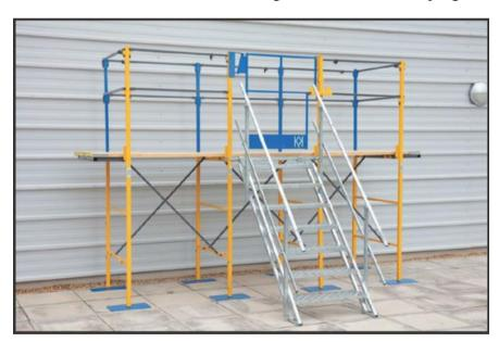
13. The invention claimed in EP 738 is a safety feature which concerns the horizontal rails on the working side. In the photograph they are above the wooden platform and on the side of the trestles adjacent to what looks like a metal door. These (grey) horizontal rails and the (blue) uprights to which they are attached are removeable.
