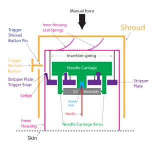
59. The G7 Applicator will not actuate unless and until the Trigger Shroud Button is depressed. The process leading up to the depression of that button, and the events that follow it are set out in the following diagrams showing the G7 Applicator at various positions.
