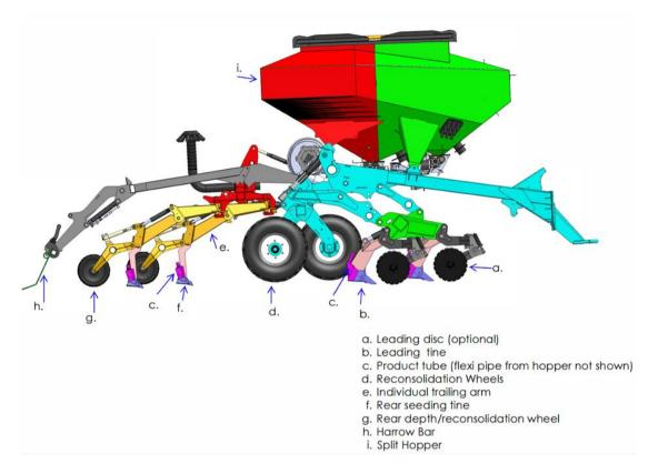
61. The trailing arm assemblies, including the rear seeding tine (f) and the rear depth/reconsolidation wheel (g) (the soil levelling means of claim 8), are pivotally attached to the frame by horizontal pivots. These allow each of the rear tines to follow the trench and disturbed soil created by the corresponding leading tine (b) even when the drill is towed by the tractor along a curved path at the end of a field (the "headland"). This is illustrated in the following diagram from the PPD:
