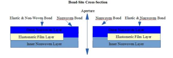
The elastomeric film layer is the stretchable layer of the claims.
