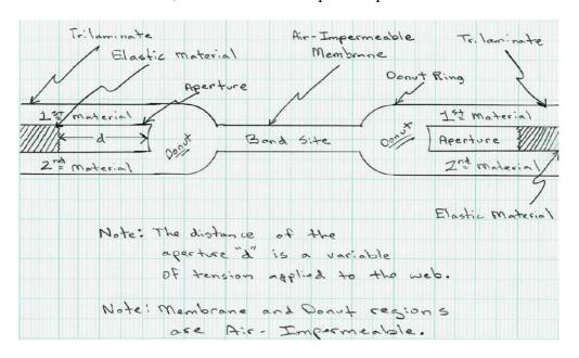
26. Instead of the outer and inner layers fusing to form a grommet, they fuse into a thin single layer at the centre, impermeable to air, where the stretchable layer had disintegrated. Peripheral to the central single layer there is a thicker single fused layer, a 'donut'. Mr St Quintin said that notwithstanding Mr Brinkley's notation, in
