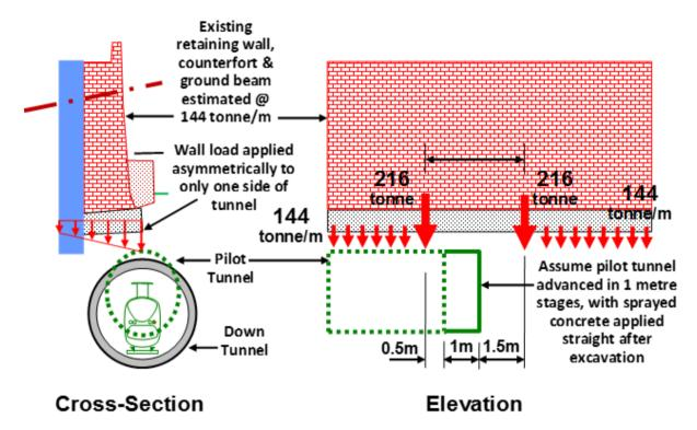
(The 0.5m and 1.5m figures are not explained in the report. However, in unsolicited emails received after the hearing Messrs Elliff and Woods appear to be in agreement that the earth ahead of the advancing tunnel will be disturbed or "relaxed" by the excavations and cannot support the weight of the retaining wall. I do not understand Mr Woods to agree the dimension.)
