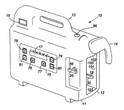
The removable canister slides into the aperture on the right.
