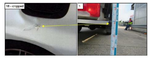
3.1.11 This damage to the Mercedes can only have occurred when the Mercedes was stationary because there are no marks leading rearwards away from the area of maximum deformation. This damage could be consistent with the two vehicles contacting each other but it is not consistent with the Mercedes moving forwards as described in the collision circumstances.
