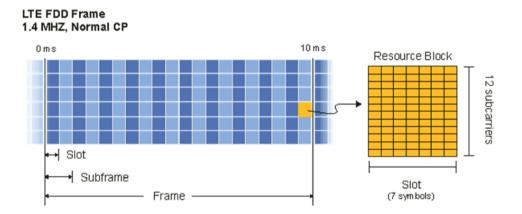
286. The allocation is by done by means of "resource blocks". The rectangle shown on the left divides available resources by time along the x-axis and by frequency along the y-axis. In the time dimension, transmissions are organised into 10ms "frames". Each frame is subdivided into 10 "sub-frames". Each sub-frame consists of 2 slots of 0.5ms. Each slot consists of 7 "symbols". In the frequency dimension, transmissions are
