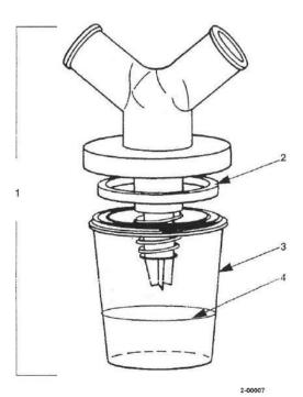
90. Although water traps are good at removing water that has condensed and drained into them, they do not remove condensed water that has collected elsewhere in the circuit. They also do not reduce the relative humidity of the
