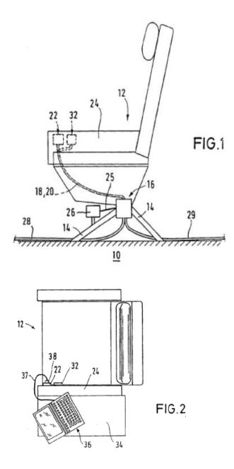
34. Figures 1 and 2 (above) showed side views and plan views of the voltage supply arrangements. Figure 1 showed a supply device (16) under the seat, connected by a signal line (18) and a supply cable (20) to a socket (22) in the armrest of the passenger seat. Figure 2 showed a connected device (specifically, a laptop) (36). The armrest also had a display device (32) to indicate the operating state of the supply device.
