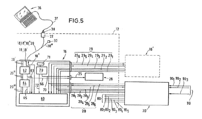
43. Figure 5 (above) showed an arrangement in which a central voltage source (30) was connected to several supply devices (16, 16'). The short circuit detector (62) and the
