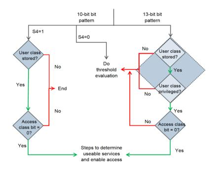
60. Both experts accepted that in Figure 4, only privileged classes need to have an access class bit. This is because these are the only classes capable of bypassing the lottery. Dr Irvine also accepted that if one did want the flexibility of making any normally privileged class into a privileged class then that normally privileged class also needed to have an access class bit.
