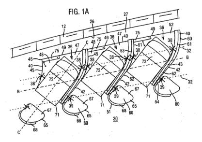
64. The figure shows three adjacent seat units forming part of a column. Each seat unit has a front end (51), and rear end (52) and two opposing sides (53) and (54). At the front end there is an ottoman (65). Along one side of each seat unit is an upstanding
