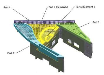
114. The rear console houses cabling and power for the actuators and lighting equipment in some seat units and also houses the power for the in-flight entertainment. The part marked Part 1 is forward of the passenger when seated and houses the life vest or is used for stowage. Part 2 is aft of the passenger when seated. Part 3 comprises elements A and B. Element B is a recessed portion. Part 4 is a decompression grille.
