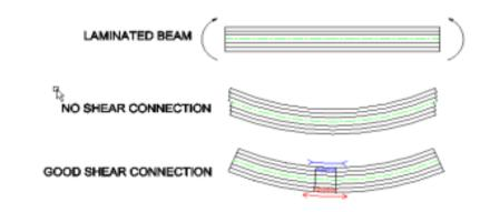
With no shear connection, one can see how the laminates tend to debond creating a ragged end of separate layers, whereas with good shear connection, the laminates stay bonded in a neat line. The capacity of the material to do this is called inter-laminar shear strength.
